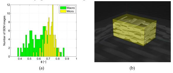
**Figure 1:** Distributions of micro- and macroscopic volume fractions in the textile specimen yield by the image analysis of scanning electron microscopic data (a). Microtomographic data treatment for the geometrical reconstruction (b).
